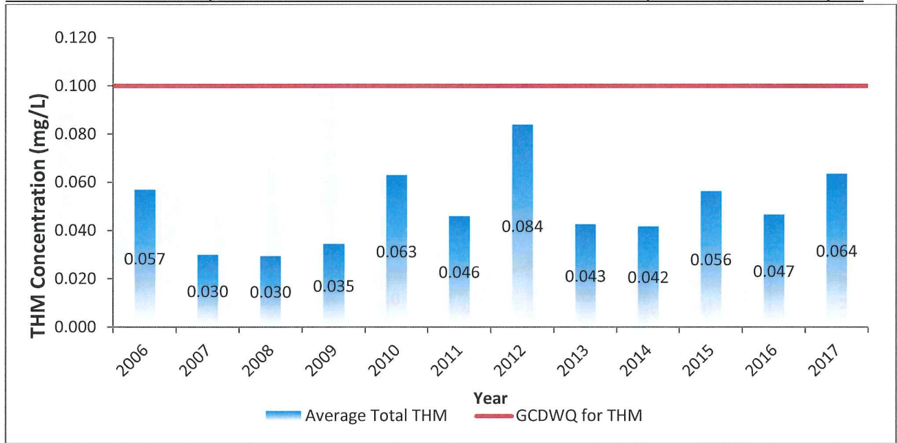
Figure 5. DLC Okanagan lake source trihalomethane (THM) data collected 2006 – 2017. Average Total THM values relative to the Guidelines for Canadian Drinking Water Quality (GCDWQ).
