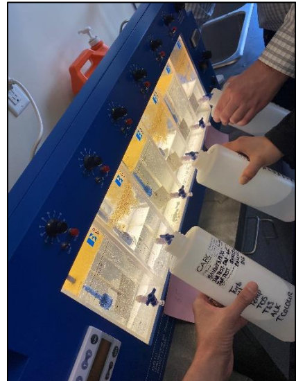
Image 3: Jar Testing to evaluate coagulation chemistry.
