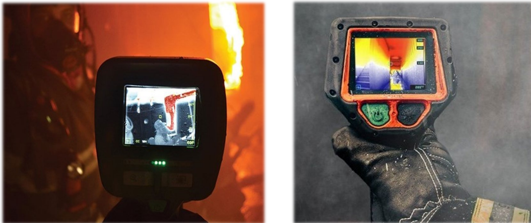
The images show a third generation TIC (10 years+) on the left and a fifth generation TIC (new) on the right.
