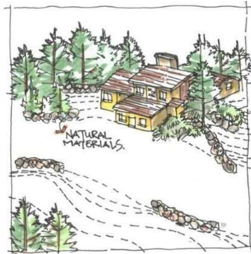
This drawing provides an example of appropriate uses for retaining walls that are low in profile, use natural materials and are broken up into sections to reflect the natural terrain.
