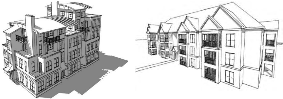
Undesirable Multiple-unit configurations – No building articulation, featureless rooflines, no creative use of materials
