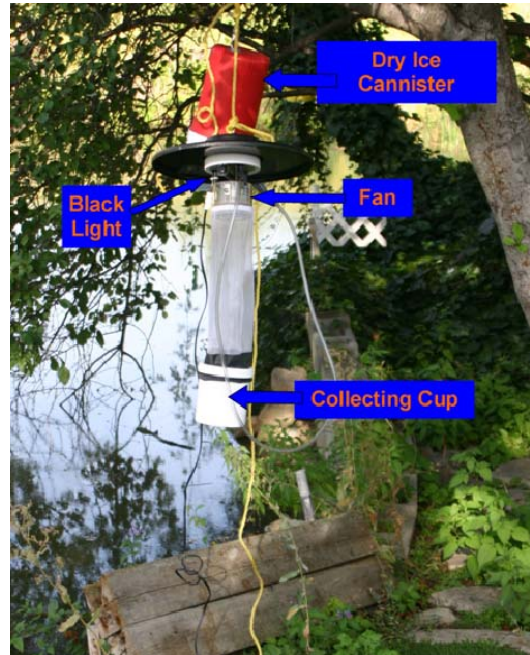
Figure 2. CDC mosquito black-light trap with dry ice canister.
